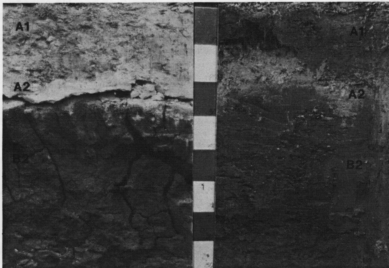
Plate 6.3 Brumby soil structure dry (left) and wet (right); note the prismatic structure when dry and essentially massive structure moist. The bleached A2 horizon is hard setting when dry and becomes a structureless slurry when wet.
