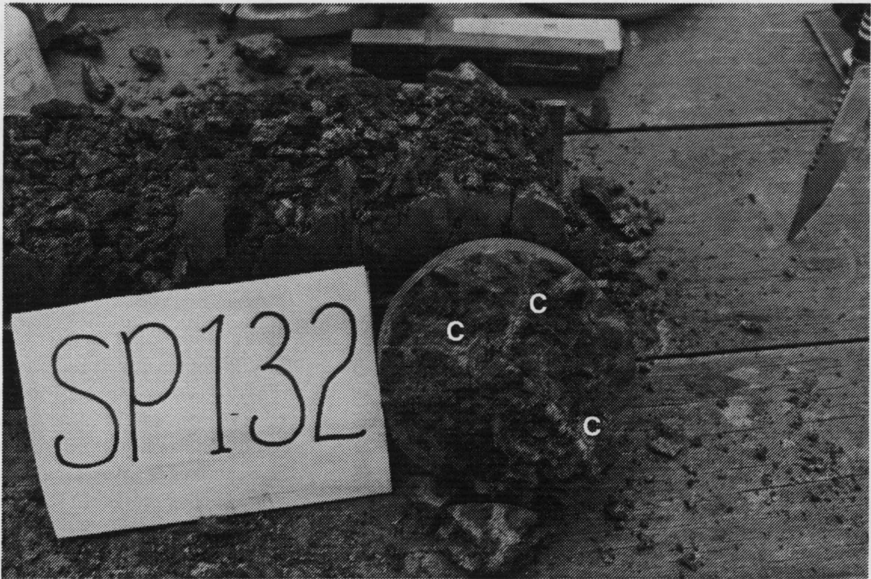
Plate 6.12 View of the subsoil of soil profile 132, Woodstock soil profile class, showing thick clay coatings suggesting clay translocation in duplex soils in the Launceston Tertiary Basin (note 'Y' shaped cracks coated with clay, indicated with letter 'C', 524600E, 5363750N, AMG).
